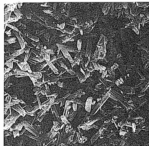
Figure 56.28: Structure of set and hardened gypsum (scanning electron micrograph). The structure shown in the photograph of set hemihydrate plaster is typical of re-hydrated gypsum: the characteristic features are determined by needle-like particles that interlock and intergrow and by the high degree of porosity (2000 ×).
